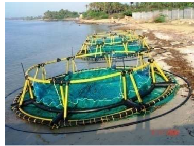
Fabricated sea cage ready for launching
